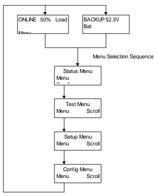
The Mode Display will be shown after the unit's first power up diagnostics have been run, or when it is selected by stepping through the menu selections.
